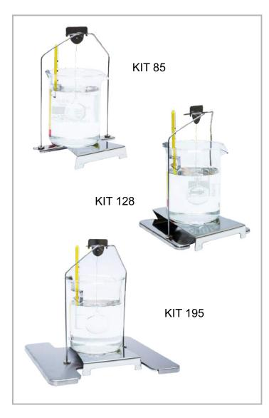
The density determination kit of solids and liquids is inteded to cooperate with laboratory balances featuring weighing pans with dimensions ø85 and ø100 mm [KIT85], weighing pan 128×128 mm [KIT 128] and weighing pan 195×195 mm [KIT 195].
