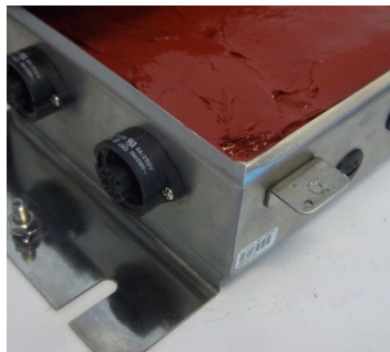
Insulated electronic PCB's with 300 °C RTV materials and military type connectors
