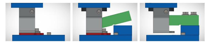
Thanks to support plates enable installation without load cell. Load cell can be replaced easily without disassembling the module. Support plates are removed up to operate as lift-up parts.
