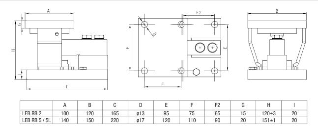
Tank weighing system with 3 load cells
