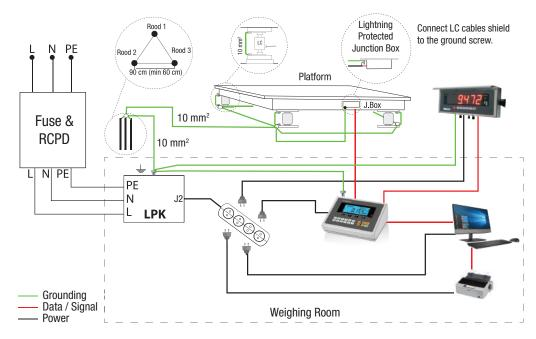
With a dedicated grounding, LPK connection to a scale with analog load cells.
