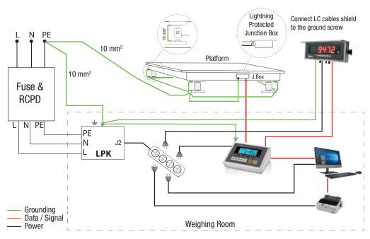
With a facility PE grounding, LPK connection to a scale with analog load cells.
