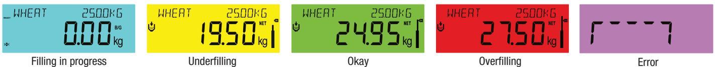
The operator follows the operation is done in tolerance by multicolor display. Continuous under filling or overfilling means that there is a mistake at the parameter entries of the controller, and this mistake must be corrected to increase system efficiency. For example, continuous overfilling (red display) may mean that the coarse feeding is made more than necessary.
