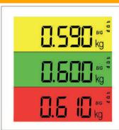
**Over-Under Checkweigher** Classifying by weight or count supported by color changing display and +/- bar.
